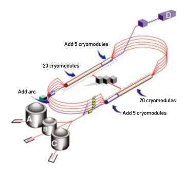
Figure 5.3. Elements of the CEBAF upgrade. Increasing the beam energy at CEBAF from 6 to 12 GeV requires upgrades in four areas: (i) additional accelerating power, (ii) stronger magnets in the recirculation arcs, (iii) an upgraded cryoplant, and (iv) one additional recirculation arc. The higher-energy electrons can be directed to a new experimental area, Hall D.
