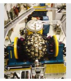
View of the gamma detector array GAMMASPHERE which was used in the experiment described below.It consists of about 100 Ge crystals used for the high-resolution detection of gamma rays from nuclear reactions.
