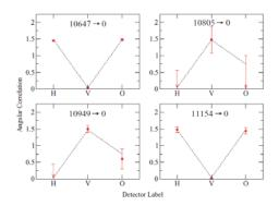
Angular Correlation of four of the observed states. Gamma-ray excitation by a linearly polarized beam is one of the only definite methods of determining the spin-party of a state. The geometry of the detectors shown in the figure below maximize the differences in intensity seen for the different possible de-excitation modes (M1, E1, E2).
