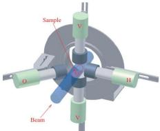
The experimental setup consisted of 4 60% High Purity Germanium (HPGe) detectors placed in a geometry conducive to the determination of the spin and parity of the observed states. The target was 16 grams of 99.5% enriched  $^{26}$ MgO.
