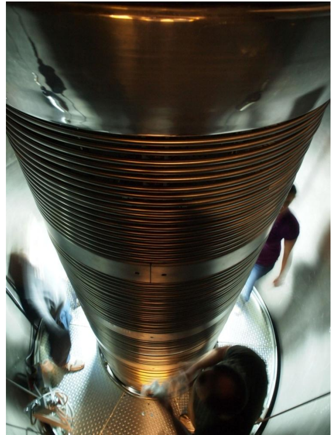
Inside the accelerator, as seen from the upper access way. The moveable maintenance platform can be seen in position at bottom of picture.
