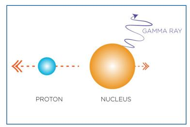
When a nucleus emits a proton (or neutron), the residual nucleus recoils in the opposite direction. The Doppler shifts of gamma rays emitted from the nucleus can be used to determine the speed of the nucleus and, hence, the kinetic energy of the proton (or neutron). Image credit: Erin O'Donnell
