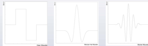
Different Wavelets (Ψ) used in the CWT analysis; best results are obtained with the Morlet Wavelet
