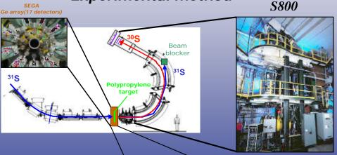
The energies of excited levels above the proton threshold of the nucleus 30\$ have been measured in a neutron removal experiment in inverse kinematics at NSCL using the \$800 Spectrograph in combination with the Segmented Germanium Array (\$eGA).
