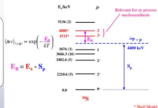
The situation for the <sup>29</sup>P(p, γ)<sup>30</sup>S reaction is shown in the figure. Two levels above the proton threshold are predicted to contribute to the total reaction rate.
