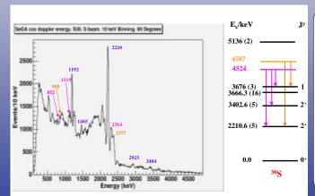
The Doppler corrected photon spectrum associated to the identified <sup>30</sup>S nuclei is shown in the figure. In addition to the known lines (blue), several gamma lines can be identified as transitions from two levels located above the proton threshold:
