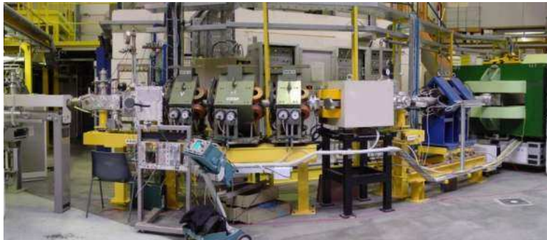
ARES at Louvain-la-Neuve Used to measure ^{19}\text{Ne}(p,\gamma)^{20}\text{Na}
