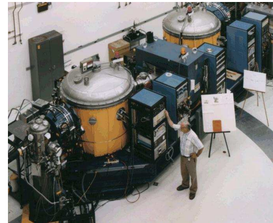
FMA at ANL ATLAS Used to measure ^{18}\text{F}(p,\gamma)^{19}\text{Ne}
