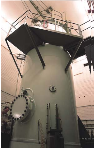
A 5 MV Pelletron with ECR source in terminal.
