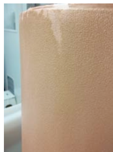
Figure 2: Copper growing on a mandrel that has been remachined at the Davis Campus
