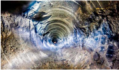
Figure 5: This diamond drill borehole is only eight inches in diameter but in Matt Kapust's photo it looks like a tunnel. The photo also reveals information about rock stresses.
