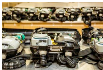
Figure 8: Self-contained breathing apparatus units are prepped for use by the Emergency Response Team
