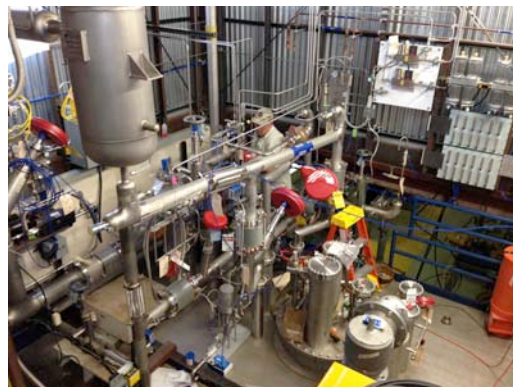
Figure 2: LBNE prototype cryogenic system
