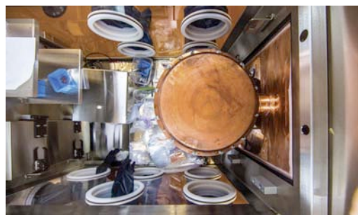
Figure 5: A copper cryostat, as seen from above, will hold the extremely sensitive detector strings. This cryostat is a prototype of the ultra-pure copper that will be used in the actual module
