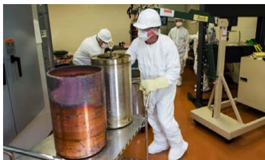
Figure 5: Machinist Randy Hughes maneuvers a cart carrying a 200-pound cylinder of copper recently quenched from a stainless steel mandrel (right)
