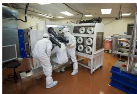
Figure 4: Researchers Wenqin Lu (LANL) and Florian Fraenkle and Matthew Green (Univ. of North Carolina) work on a string of germanium detectors in a glovebox
