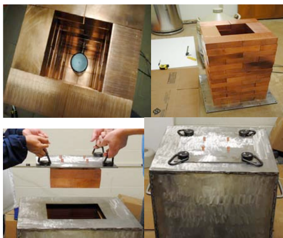
Figure 3: Detector (upper left), copper shield (upper right), lid cover (lower left), and radon exclusion box (lower right)
