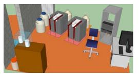
Figure 3: Illustration of Berkeley Lab Low Background Counting Facility at the Sanford Lab Davis Campus. Currently, only one detector is being installed but the space can accommodate a second detector
