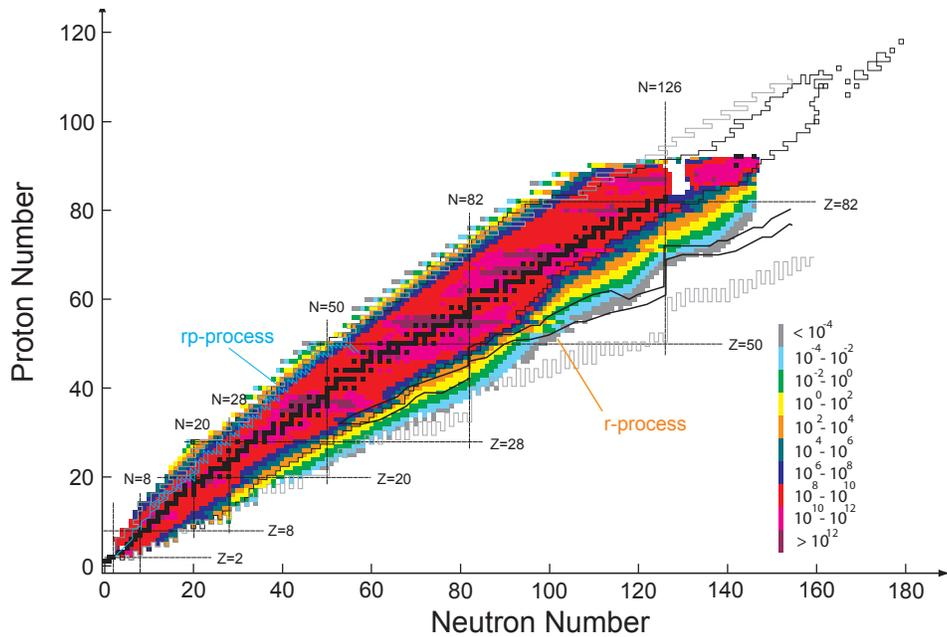
**Figure 7.3:** Contour map of re-accelerated beam intensities for all isotopes calculated based on a 400 MeV/nucleon 400 kW primary beam. The plot includes beams produced by ISOL and those extracted from a gas-stopping cell; the optimum yield is chosen for each case. For reference the r- and rp-process paths are shown, as well as the projected location of the proton and neutron drip lines. The rates are given in particles per second.
