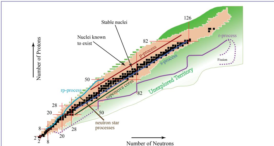
**Figure 3.1:** Lines on the chart of nuclides delineate schematically some of the important nuclear reaction sequences occurring in the universe. RIA can create most of the unstable nuclei participating in these processes. Note that the dashed line at the right end of the r-process path is not meant to indicate the actual path of the process, but to indicate that material is being recycled through fission of the heaviest elements.
