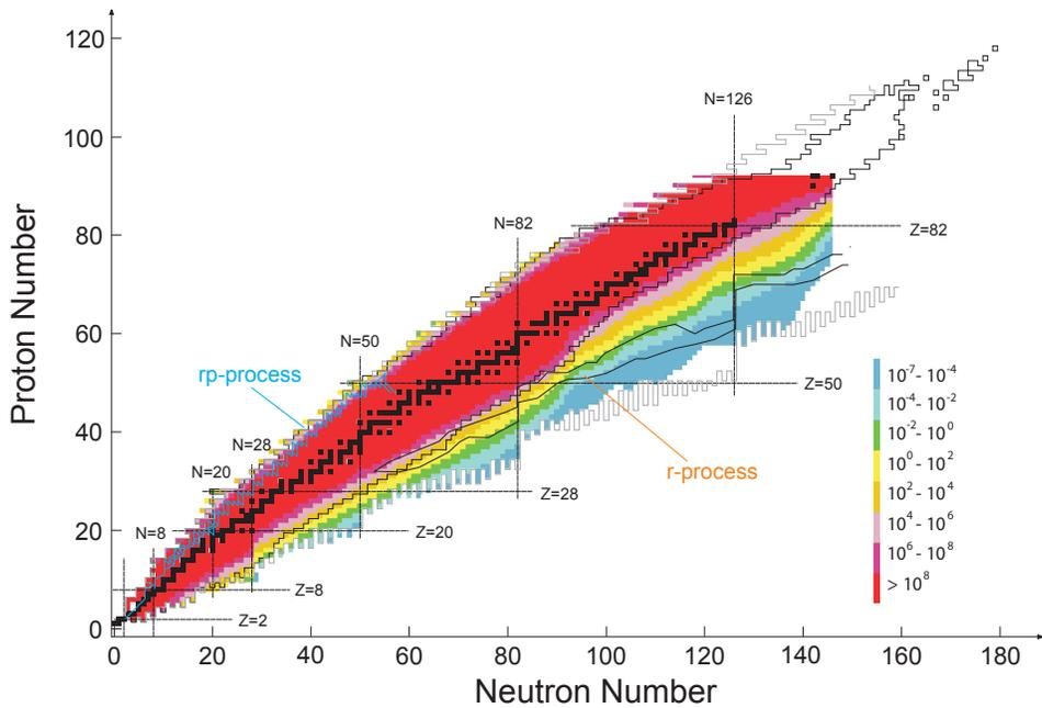
**Figure 7.4:** Contour map of isotopes calculated for fast beams produced with a 400 MeV/nucleon 400 kW primary beam. The plot includes beams produced by either fragmentation or in-flight fission; the optimum yield is chosen for each case. For reference the r- and rp-process paths are shown, as well as the projected location of the proton and neutron drip lines. The rates are given in particles per second.
