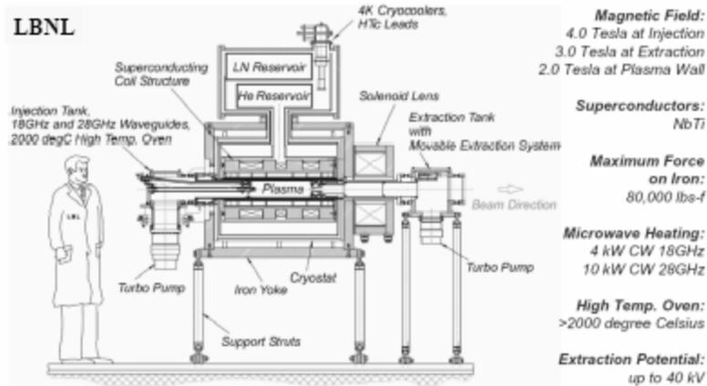
7 Early test at 28 GHz yielded  $> 8 \mu\text{A}$  of  $\text{Bi}^{30+}$  ions, ~RIA specs for 400 kW
