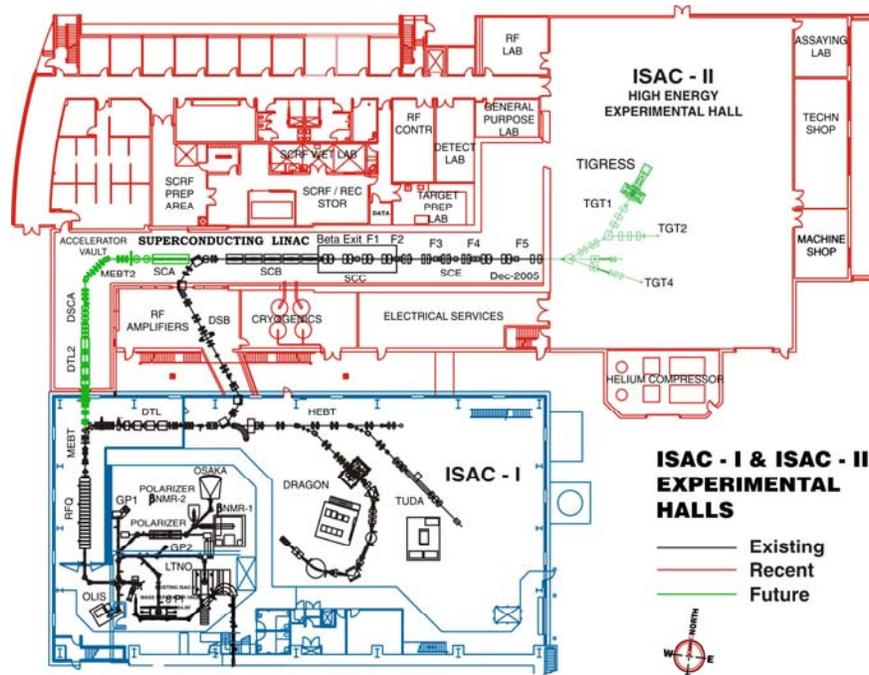
Figure 3.1: Layout of the accelerators and experimental stations in the ISAC facility.
