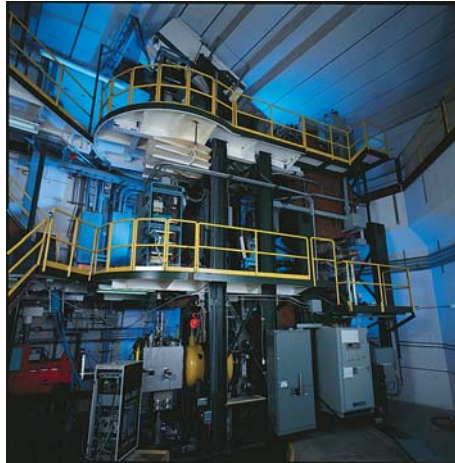
The S800 magnetic spectrometer at the NSCL used in the measurement of the Gamow-Teller distributions via the (Hydrogen-3, Helium-3) reactions.
