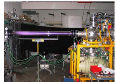
He beam in extended window-less Nitrogen gas-target.
