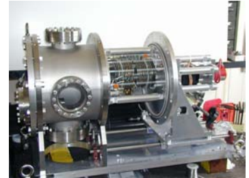
Array of twin-ionization chambers used in the study of the \beta -delayed \alpha decay of ^{16}\text{N} .
