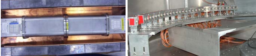
Clover Detector (left) and Si detector (right) arrangements for p-process cross section studies by activation and elastic scattering measurements.
