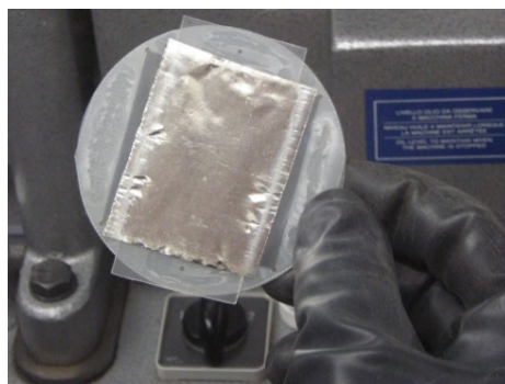
Photograph of a pure lithium metal target prepared for this work. The metal reacts rapidly with air or moisture and must be prepared and handled with great care in an inert atmosphere.
