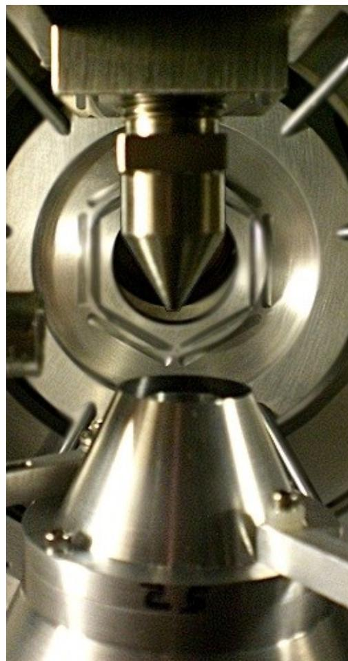
The JENSA jet nozzle and gas receivers inside of the target chamber.
