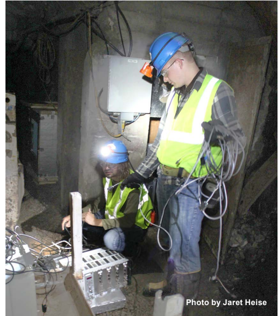
Notre Dame University physicist Andreas Best (kneeling) and graduate student Karl Smith set up a counter to detect neutrons on the 4100 Level.
